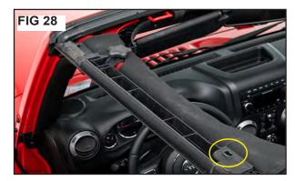
Line up the door surround "C" attachment holes with the vertical holes in the roll bar. Slip the front long knob through the hole in the front door surround (FIG25). Tighten the knob securing the front door surround (Fig 26).
