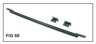
Locate the Tailgate bar and brackets (FIG 88). Locate the driver's side bracket. With the lip to the outside of the vehicle, line up the bracket with the slot in the body tub, hook the rear portion of the bracket to the body tub and roll the bracket forward until it click
