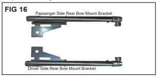
Locate the two rear bow mount brackets shown in Fig 16. Locate the Driver side rear bow mount bracket with the flat steel tab facing down and place the bracket over the door surround hole with the quick release knob facing in
