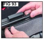
Take the Tailgate bar and orient the "C" Channel with the round seal facing down and slide the "C" Channel onto the rear window retainer as shown in FIGs 92 & 93.
