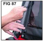
Secure the rear window zippers by pulling the two zipper sliders all the way down as far as possible in order to catch the sliders on the zipper pin. Once the zipper is caught, raise the zipper 1"-2".
