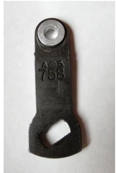
Shown here is the bushing installed into the transfer case pivot plate. There is no need at all to remove this bracket from the transfer case, like the one shown here for clarity.
