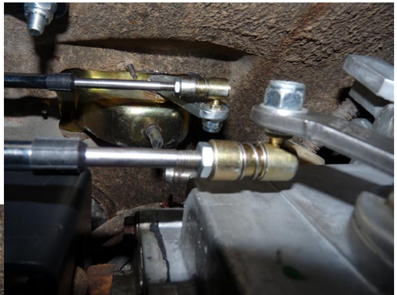
Shown here is the bushing installed into the transfer case pivot plate. There is no need at all to remove this bracket from the transfer case, like the one shown here for clarity.
