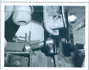
Fit M14 x 80mm bolt with flat washer through bracket lower hole. Fit 4mm thick washer to inside of bracket.
