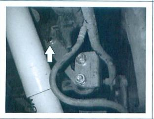
Fit tension member to chassis using M12 x 30mm bolt, nut and washers as shown.
