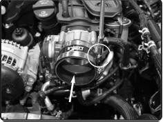
**15.** Now install the straight hose with clamps provided to the throttle body.
