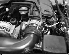
**5.** Loosen the clamp on the throttle body using 8mm nut driver.
