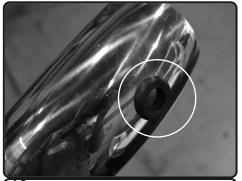
**16.** Install the provided grommet to the hole on the intake tube.
