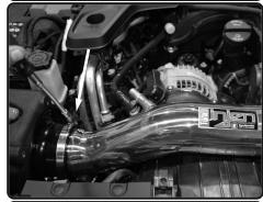
**19.** Tighten the clamp on the filter using 8mm nut driver.
