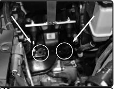
**13.** Make sure the stand off studs are seated in the OEM grommets properly.
