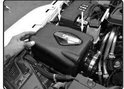
**14.** Powerslow box installed and seated properly.
