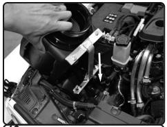
**12.** Install the powerflow box assembly into the vehicle.
