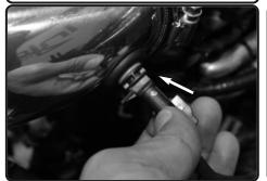
**20.** Re-install the temperature sensor to the grommet on the intake tube.
