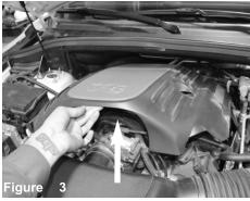
Lift up and remove the engine cover.
