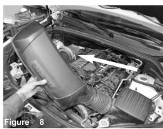
Now lift up and remove the complete stock intake tube.
