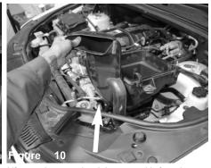
Lift up and remove the air box assembly from the vehicle
