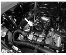
Now tighten the clamp on the throttle body using 8mm nut driver. Secure and tighten.
