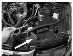
Line up the hole on the bracket of the heatshield to the location where the bolt was removed from figure 6. Reuse the O.E. 10mm bolt to secure the heatshield bracket to the radiator support.
