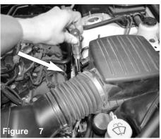
Loosen the clamp on the air box.
