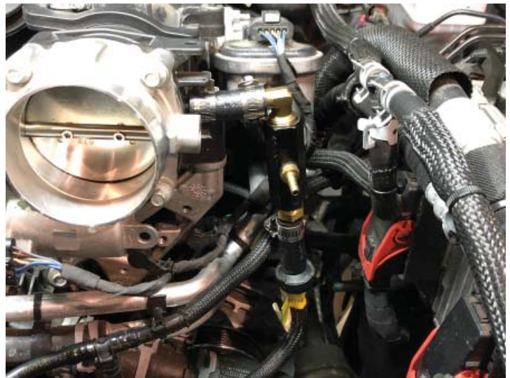
Vacuum Manifold Installed
