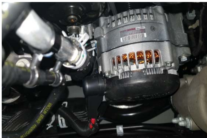
Plastic Cover Installed Over Power Wire
