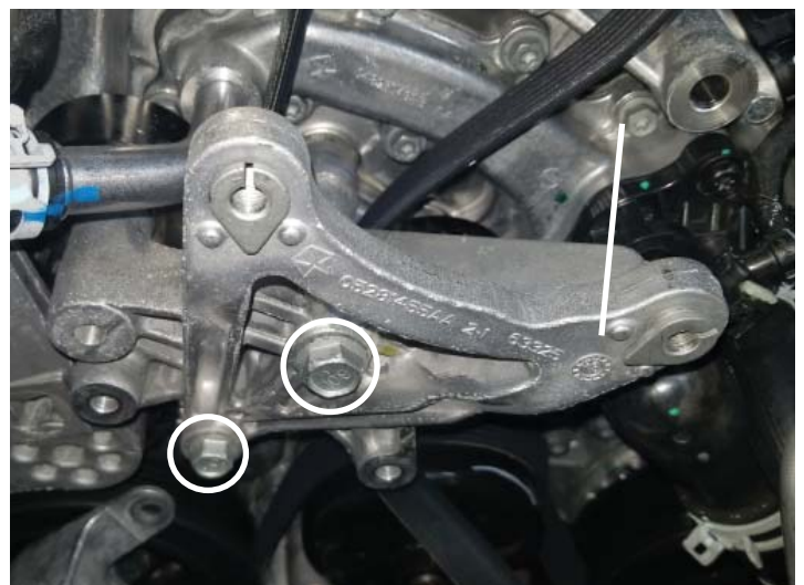
Alternator Bracket Bolts
