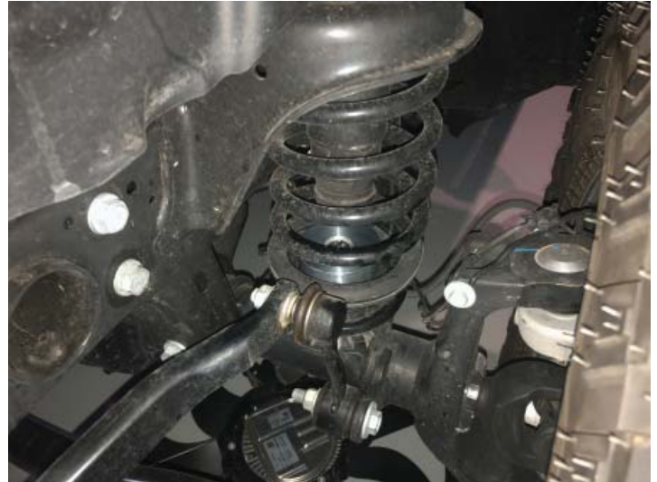
Bump Stop Installed
