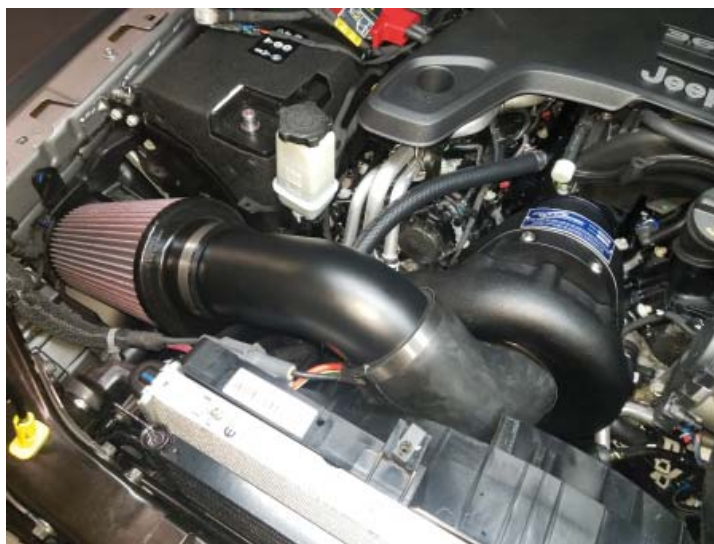
Air Inlet Installed
