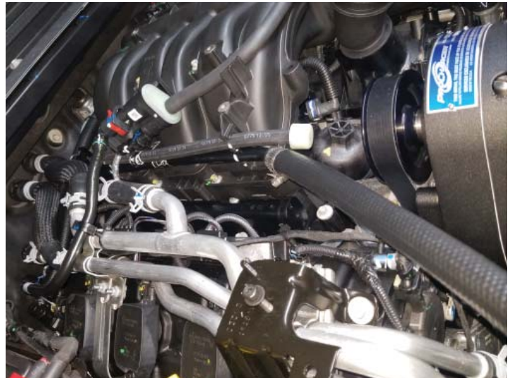
Hard PCV Line Trimmed
