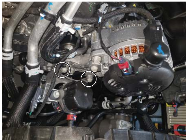
Remove Air Pump Bolts
