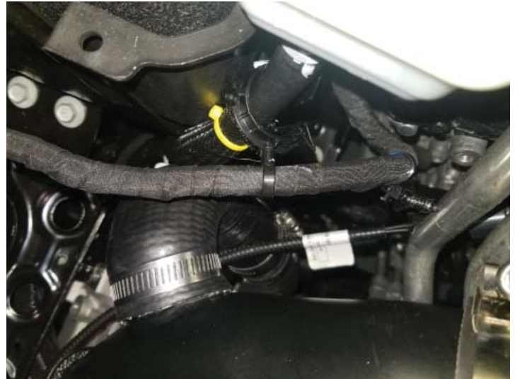
Moulded Rubber Hose Installed
