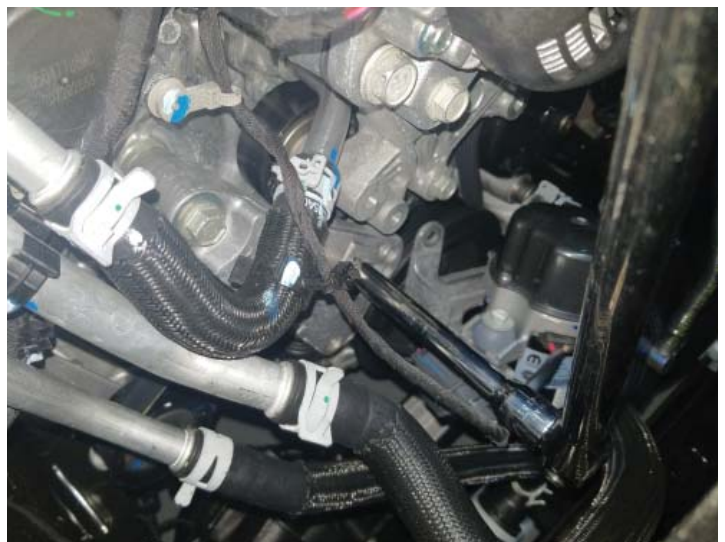
Compress the Tensioner and Remove Belt
