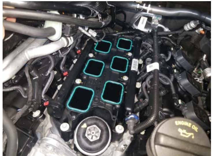
Intake Manifold Removed
