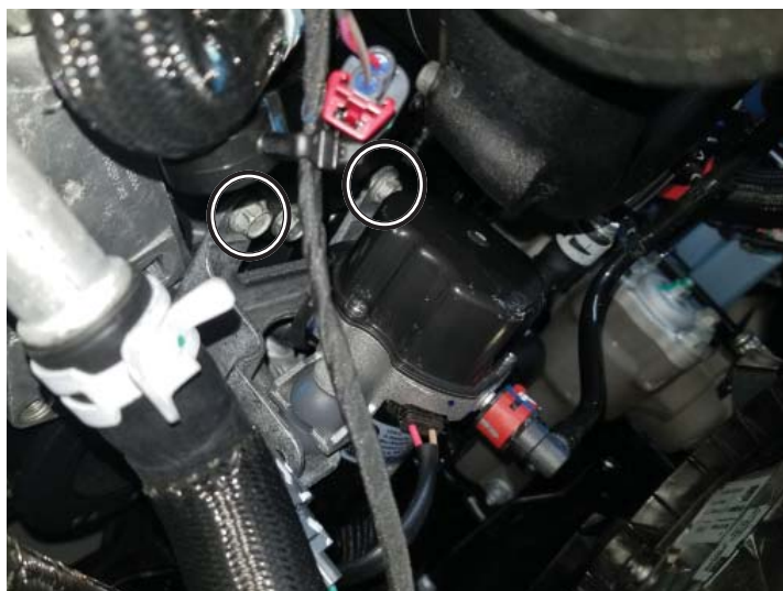
Air Pump Mounted
