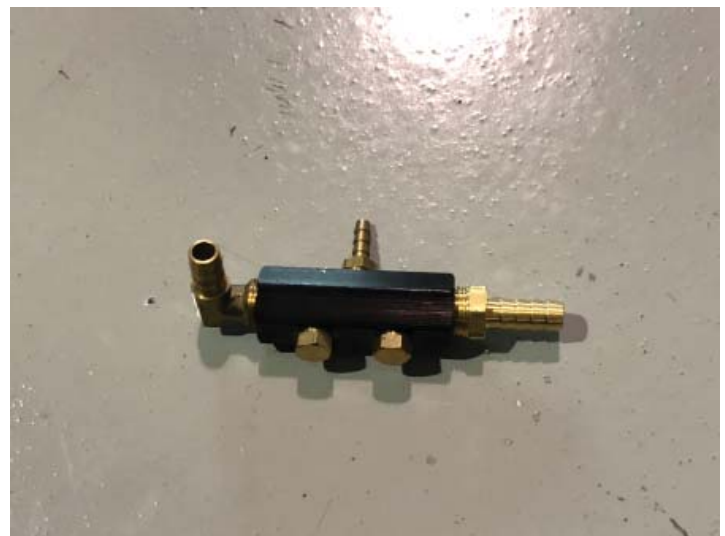
Vacuum Manifold Assembled
