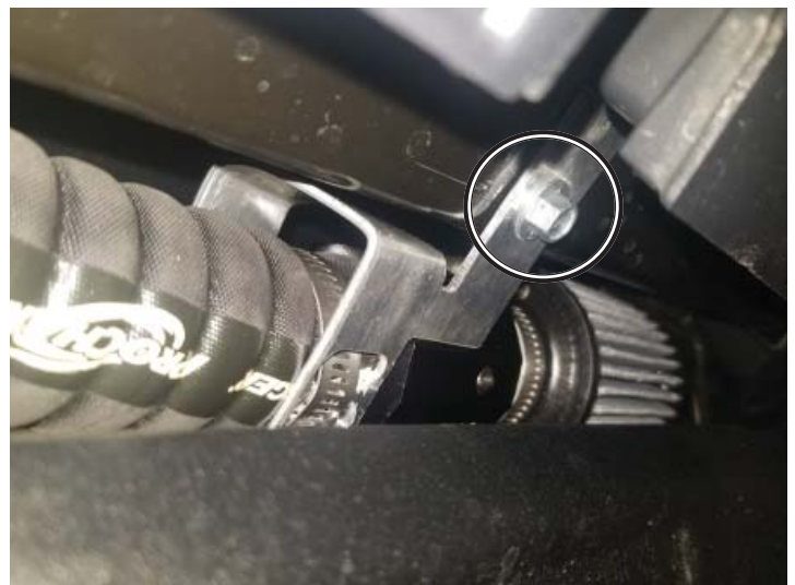
Surge Valve Installed
