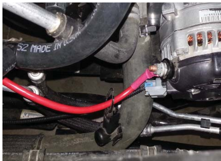
Harness and Power Wire at Alternator
