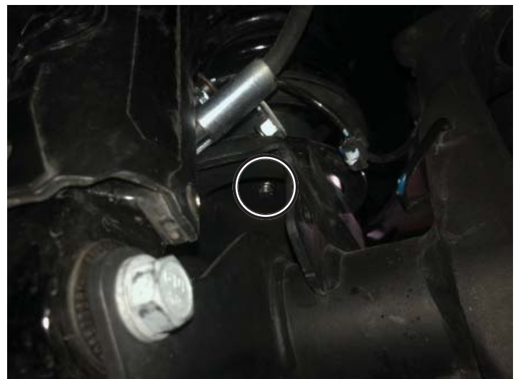
Bump Stop Nut Installed
