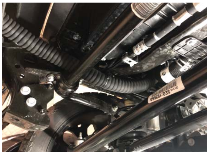
Surge Tube Routed
