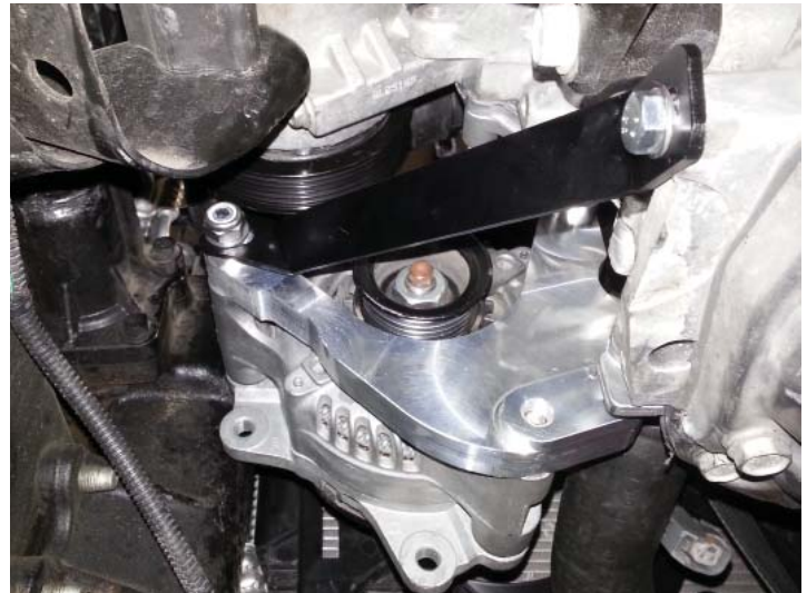
Alternator Brace Installed
