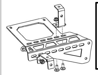
When bracket or any accessory is mounted on the top of the brackets the windshield will <u>not</u> be able to be folded down. If the bracket or any accessory is mounted on the side there is a possibility that the windshield may not be able to be folded down. Bracket is not intended for a Light Bar.
