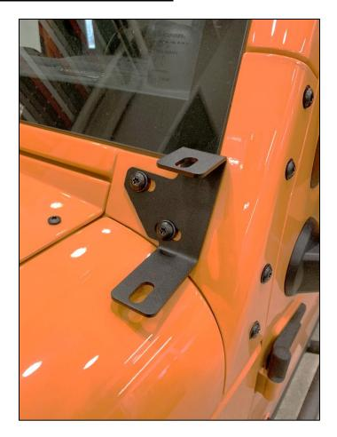
When Lower Light bracket is mounted the windshield will <u>not</u> be able to be folded down.
