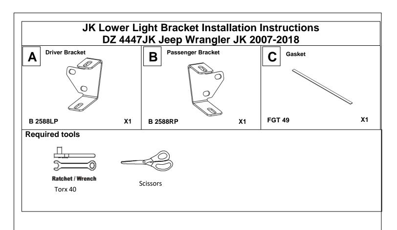
First cut the Gasket (C) into 10 pieces. Lengths are 2 7/8", 2 1/4", 1 3/8", 1", 5/8". There will need to be two of each length.
