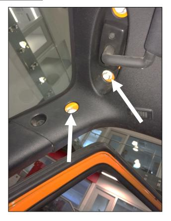
Attach the bolting block (B) to the grab handle (A) using screws (E) and binding posts (F). The larger hole of the bolting block should be facing down. Fully <u>Tighten at this</u>
