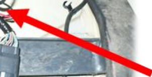
Run the harness wires behind the large metal plate seen here on the side wall so they pop out over where you had removed the Driver side dash side panel. Make sure the wires aren't tugging on anything and are clear of brake and clutch pedal movement, etc.
