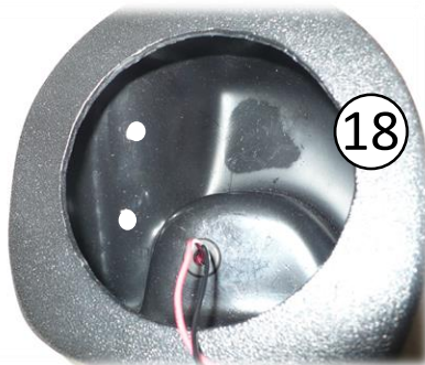
18 Good approx. locations for self-tap screws shown by white dots inside pod. May help to pre-drill but not absolutely necessary. If you do, be sure to remove any plastic shavings on the other side from drilling through so you get a nice fit on the plastic windshield piece on the Jeep.
