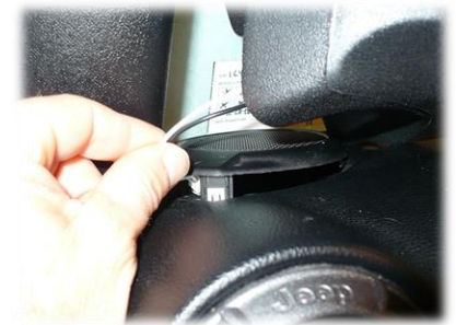
2015-2018 Wranglers: Leave enough wire coming out in the shown area and snap tweeter covers back in place. Put pod in place and pull all excess wire through. The idea is to have enough wire to hold the speaker up and connect to it easily once pod is affixed to vehicle. Excess wire goes below in tweeter cavity.
