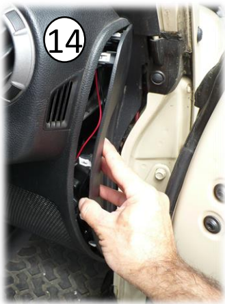
14 Snap side panel back in place.
