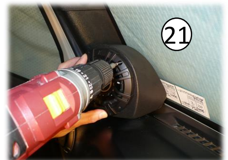
21 Situate speakers and grilles with logos how you like and screw speakers in place with the screws that came with your speakers. Most of the time the screws will grab and make their way through the plastic. You can pre-drill some holes with a small drill bit if needed.
