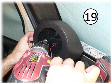
19 Find the pod's sweet spot. You'll find the pods kind of lift and slide up the Jeep pillar slightly to find the correct position. Hold pod in place with one hand and run the upper self-tapping screw through the pod and into the plastic pillar piece until just snug. Run the lower screw in next.
