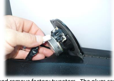
Disconnect and remove factory tweeters. The plugs can drop down in the cavity, you won't use them for this install type. If one of those wires (Driver side) has a purple stripe , you have a "standard" system and must follow Installation #2 and need one of those wire harnesses instead. You need Pillar-Pods part #PP1518 or #PP1518-K (with Kicker speakers) to get the correct harness.
