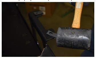
24. Place the winch into the Recessed Winch Cradle. If the winch is new, install it without the cable or rope. If the cable or rope is already installed, it will need to have a removable hook or thimble. Otherwise the cable or rope will need to be un-spooled prior to this step, and respooled after the end of the bumper installation. It is also recommended to hook up your winch wiring at this time.
