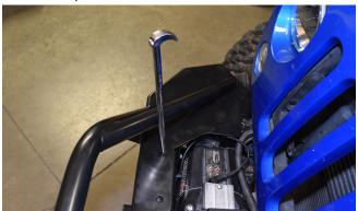
**38. Insert a provided Stainless Steel** Flat Head Cap Screw into each of the four counter-sunk holes along the top
