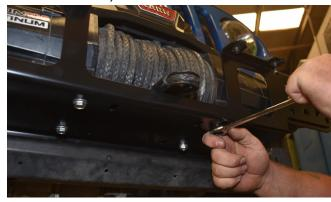
27. Pre-position the two Frame Mount Spacer Plates, between the Recessed Winch Cradle and the bumper mounting flanges on the ends of the Jeep's frame rails. Slightly loosen the previously-installed Nut Plate bolts, if necessary, to allow necessary movement of the Cradle. But keep the Nut Plate bolts tight enough to hold the Spacer Plates in place, once positioned.
