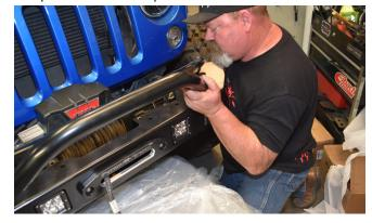
**33. There are floating bolt plates** pre-installed inside the Bruiser bumper. These bolts interface with the four large bolt holes on each of the two mounting flanges on the ends of the Jeep's frame rails. The bolt plates are "floating", that is, they can move around slightly, in order to accomodate slight variations in the Jeep manufacturing tolerances. However, this can make it somewhat tedious to get all 8 mounting bolts started into their corresponding bolt holes.
