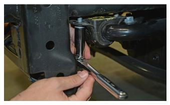
**12. Insert the mount flange of** the vacuum pump relocation bracket between the swaybar bushing block and the underside of the driver side frame rail. Reinstall and re-tighten the two swaybar bushing blocks.
