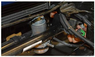
**13. Loosen the two bolts that** hold the sway bar bushing block to the underside of the passenger side frame rail, and insert the swaybar spacer in between the swaybar bushing block and the frame rail.
