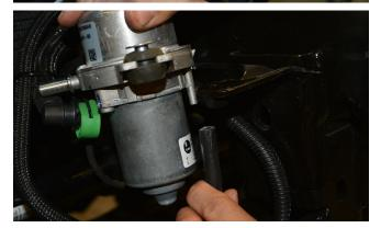
**8.** Disconnect the vacuum pump's electrical wire pigtail from the vehicle wiring harness by separating the connector.
