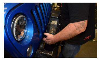
**25. Install the four mounting bolts** that came with your winch, through the bottom of the Recessed Winch Cradle, into the mounting nuts in the winch.
