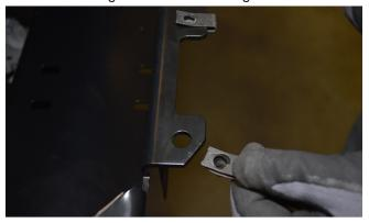
**23.** A rubber mallet or soft dead-blow hammer may be needed to properly seat and position the clip-nuts.
