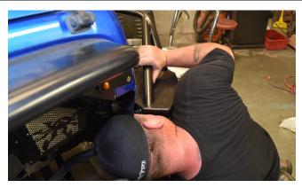
34. The best strategy is to first try to get one nut threaded on, on either side of the bumper, to start. Once there is at least one nut started on either side, it will be easier to coax the remaining threaded studs through their corresponding bolt holes.
