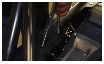
**39.** Use a wrench to final-tighten the flat head cap screws. Note that stainless steel is a softer alloy than the hardened steel of the clip-nut, and it may gall or strip if cross-threaded or over-tightened. Do not over-tighten.
