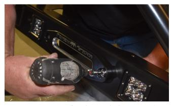
31. With the help of a friend, move the bumper (and preinstalled skid, if desired) into position close to the front of the Jeep. A padded surface to set the bumper close to the Jeep is helpful. Thread the end of the winch rope (if present) through the fairlead. Also make sure the wiring pigtails for the LED lights are positioned out of the way, so they don't get caught between bumper mounting surfaces.
