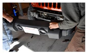
5. Remove the plastic top bumper cover. You may be able to remove the two plastic screws with a Phillips screwdriver. But it is likely they're "frozen" in place and will have to be pried up with the push-in retainer removal tool.
