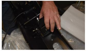
30. Install a winch fairlead (sold separately) to the front of the Bruiser bumper, using the provided mounting holes, and the hardware that was supplied with the winch fairlead.
