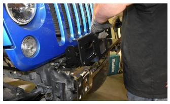
**18. Temporarily "hang" the Cradle by** the resting the right-angle flanges on to the tops of the Jeep's bumper mounting flanges.
