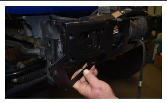
28. Note that the Spacer Plates are not symmetrical and must be oriented correctly, to match the four corresponding bolt holes in the Cradle and the frame. A spud bar or pry bar will be helpful in fine-tuning the placement of the spacer plate.
