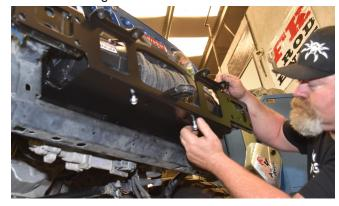
**26. Tighten the four winch bolts** to whatever specification is recommended by the winch manufacturer.
