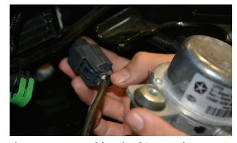
**9.** There are two rubber bushings in the mounting flanges on the vacuum pump, with steel sleeves inserted
