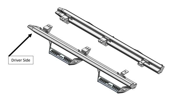
**Step.2** Starting with the passenger side step rail, install the supplied (x6) 5/16" snap nuts into the two notches in each mounting bracket.
