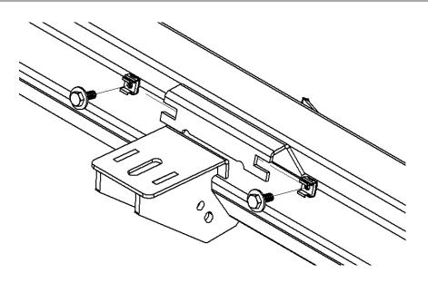
**<u>Step. 7</u>** After finial positioning, tighten all (x6) 5/16 "x  $\frac{3}{4}$ " hex bolts no more than 6 ft/lbs. torque.
