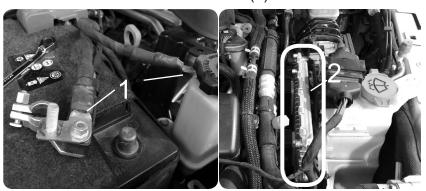
**STEP 3** - Use a flat head screw driver to press the lever lock towards the PCM. Gently lift up on the lever until you feel the lever release. (3)
