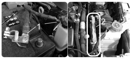
**STEP 3** - Use a flat head screw driver to press the lever locks on the ECM connectors towards the ECM. Gently lift up on the lever until you feel the lever release. (3)
