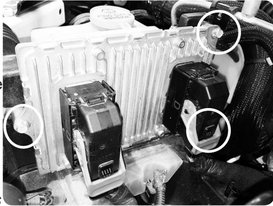
**NOTE:** The ECM connectors should be disconnected before removing the bolts.
