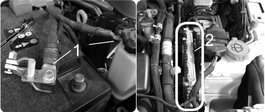
**STEP 3** - Use a flat head screw driver to press the lever locks on the ECM connectors towards the ECM. Gently lift up on the lever until you feel the lever release. (3)
