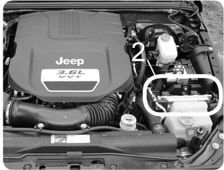
**STEP 3** - Use a flat head screw driver to press the lever locks on the ECM connectors towards the ECM. Gently lift up on the lever until you feel the lever release. (3)
