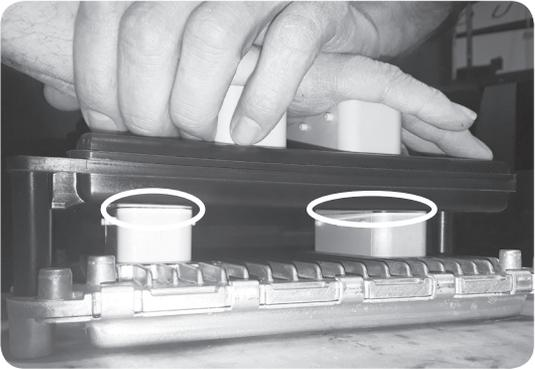
**STEP 8** - While on a flat surface, apply enough pressure to fully seat the connectors. The top of the ECM connectors should sit flush with the Pulsar enclosure.
