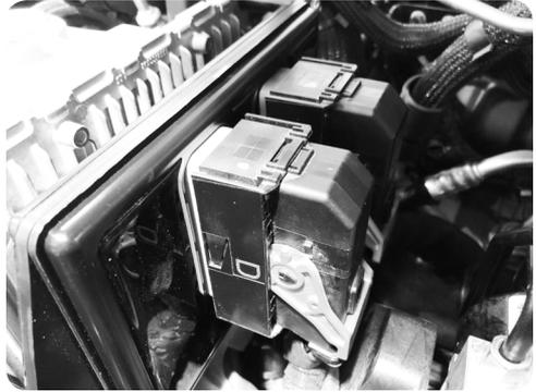
**NOTE:** Connect the gray connector first while holding it, then the brown connector after. If necessary, cut the ziptie holding the brown connector harness in place for more leeway.
