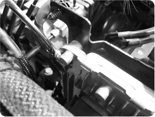
*TIP: Hold the ECM with your other hand to prevent it from falling after the last screw is removed.*
