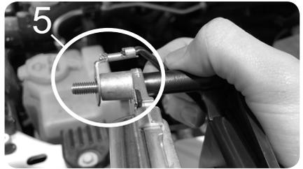
**STEP 11** - Replace the ECM and Pulsar module into the Engine bay, and line up the ECM/Pulsar bolt holes to the mount holes. (6)
