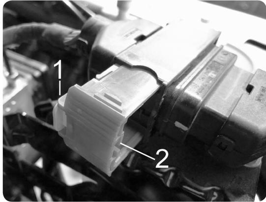
**STEP 10** - Once the red lock is completely out (2), carefully pull harness connectors apart and place the loose one out of the way.
