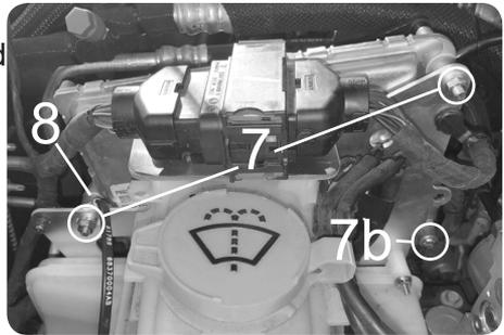
**NOTE:** The lower, inner bolt will not be connected to the bracket, only the Pulsar module. Also, use the provided Allen Wrench to tighten the bolts until snug.
