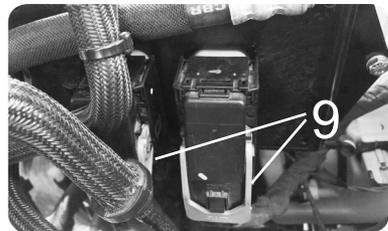
**STEP 21** - Reconnect the top harness connectors, and then lock by closing the red piece completely. Slide it back into place on the mount. (see img 7)
