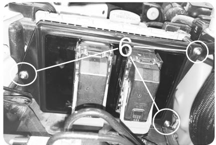
**STEP 12** - Insert the remaining provided bolts and tighten the bolts using the provided Allen Wrench until snug. (6)
