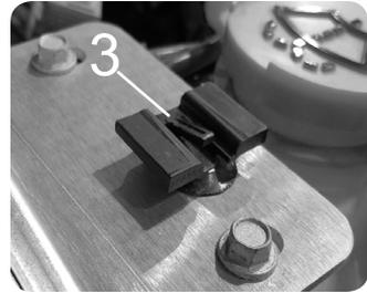
**STEP 12** - Locate and unplug all 6 plastic ziptie plugin anchors. The **Square** shaped anchors (4) can be cut if necessary, but do not cut the **Round** anchors (5).
