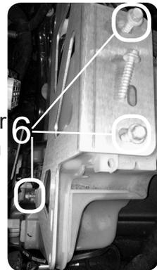
**STEP 15** - Insert three of the four stock bolts and washers as seen in image (6), and use an 8mm socket and ratchet to tighten until snug.
