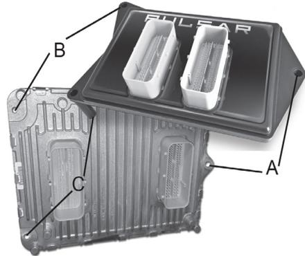
**STEP 7** - Align and insert the Pulsar's bottom side connectors with the ECM connectors.
