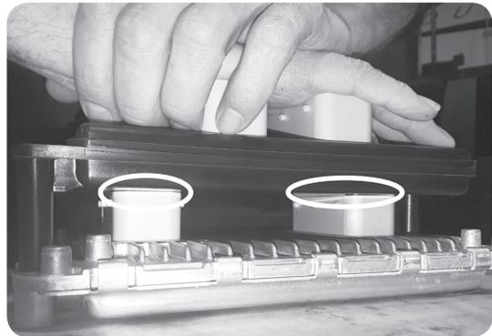
**STEP 8** - While on a flat surface, apply enough pressure to fully seat the connectors. The top of the ECM connectors should sit flush with the Pulsar enclosure.
