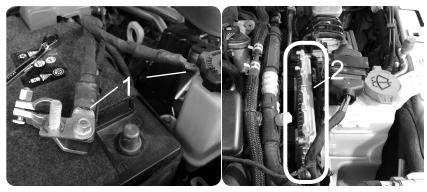
**STEP 3** - Use a flat head screw driver to press the lever lock towards the ECM. Gently lift up on the lever until you feel the lever release. (3)
