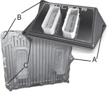
**STEP 3** - Align and insert the Pulsar's bottom side connectors with the ECM connectors.
