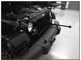
Once clips are removed, remove grille by pulling straight out and unhooking the marker lights.
