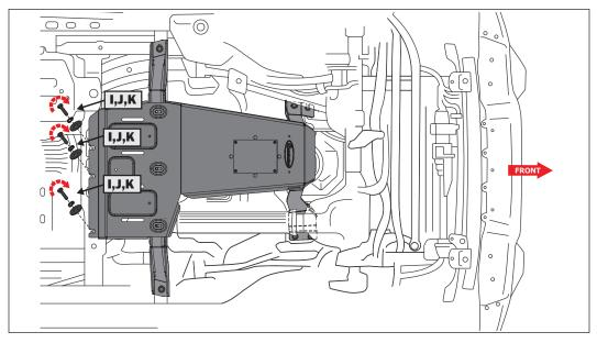
**STEP 8:** Install the (3) M12x40 bolts (I), lock washers (K), and M12 flat washers (J) into the remaining rear holes of the skid plate. Snug but do not tighten.
