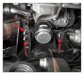
**STEP 2:** Locate the engine mounting bracket where the engine attaches to the frame. There are 3 factory bolts that you will use to install the skid plate mounting brackets.
