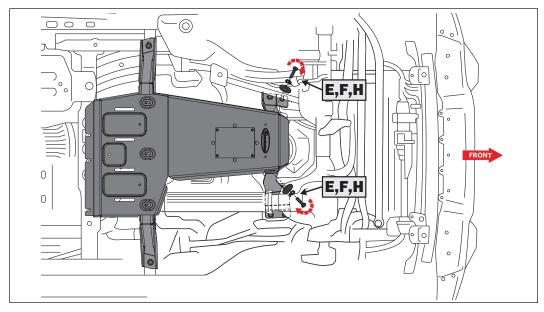
**STEP 6:** With help from a friend, lift the skid plate (A) into place and attach the front of the skid plate to the mounting brackets (B&C) with (2) M10x30 bolts (E), lock washers (H) & flat washers (F). Snug the bolts with a 17mm socket, not fully tight.
