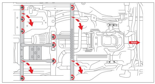
**STEP 1:** Put on safety glasses. Locate the Factory Transmission Cross brace (automatic only) and the Factory Transfer case skid plate. Remove the factory fasteners with 13 and 18mm sockets. The cross brace & transfer case skids will not be reused, but be sure to keep all of the factory bolts for re-use.
