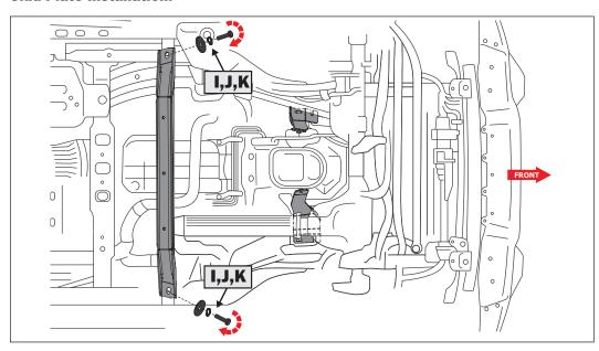
**STEP 5:** Install the Cross Brace (D) into existing holes in vehicle frame with (2) M12 bolts (I), lock washers (K), and flat washers (J). Snug but do not tighten the bolts with a 19mm socket to allow for alignment before final tightening.
