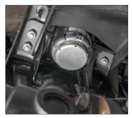
**STEP 3:** Align the Left (C) Mounting bracket with the factory bolts and install the (3) M10 X 1.50 Nylon Locking Nuts. Snug But do not fully tighten all the M10X1.50 nuts with a 17MM.
