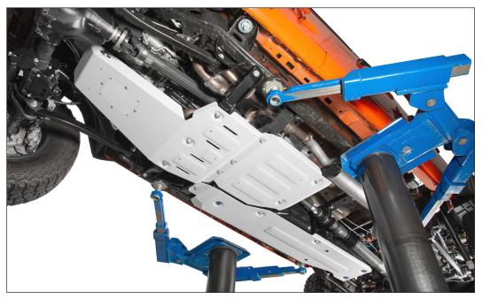
Installation is complete. This also shows the Transfer Case Skid Plate and the Fuel Tank Skid Plate (sold separately).
