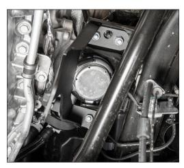
**STEP 4:** Align the Right (B) Mounting bracket with the factory bolts and install the (3)  $M10 \times 1.50$  Nylon Locking Nuts. Snug, but do not fully tighten all the  $M10 \times 1.50$  nuts with a 17MM socket.
