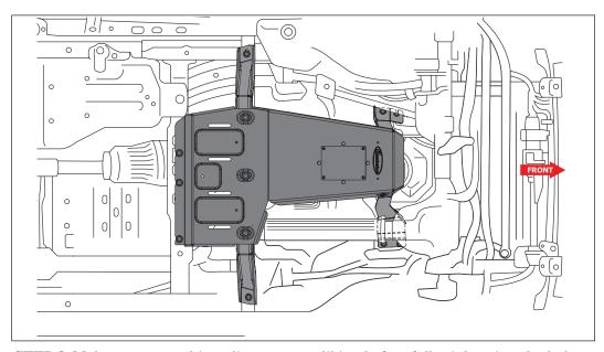
**STEP 9:** Make sure everything aligns to your liking before fully tightening the bolts. Start tightening the bolts from front to back. Tighten all M10 bolts with 17mm socket and a torque wrench to 36 ft lbs. Tighten all the M12 bolts with a 19mm socket and a torque wrench to 48 ft lbs.
