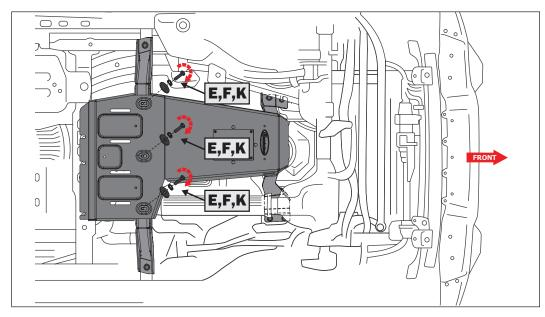
**STEP 7:** Install (3) M10x30 bolts (E) with lock washer (K), and flat washer (F) into the front 3 holes in the skid plate and thread them into the cross brace. Snug but do not tighten.
