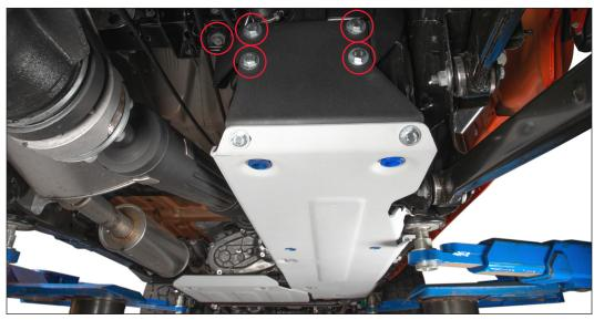
**STEP 3:** Install upper bracket (B) reusing the factory hardware. Line up lower bracket (C) to the upper bracket (B) and install (4)  $M10 \times 1.50 \times 30$ mm bolts (F), M10 lock washer (H), and  $M10 \times 30$ mm OD flat washer (G). Snug but do not tighten at this time.
