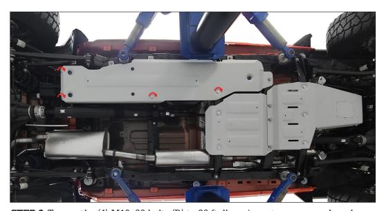
**STEP 6:** Torque the (4) M10x30 bolts (D) to 36 ft. lbs using a torque wrench and a 17mm socket. Also torque the M10 bolts on the bracket to 36 ft. lbs using a torque wrench and a 17mm socket.
