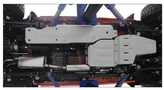
**STEP 5:** After the skid plate is fully installed tighten all factory bolts to 48 ft lbs with a torque wrench and a 18mm socket.
