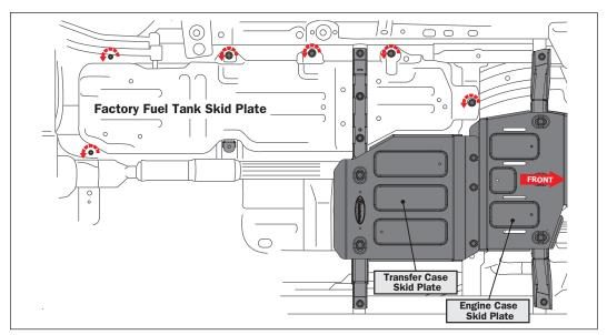
**STEP 2:** Locate the factory fuel tank skid plate. Locate and remove the remaining (6) factory mounting bolts with a 18mm socket.
