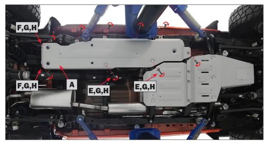
**STEP 4:** Install the new Aluminum skid plate (A) over top of your factory skid plate as shown. Reinstall the (5) factory bolts with a 18mm socket and ratchet. Also install the 2 M10x1.5x25mm bolts (E), lock washer (H), and flat washers (G) as shown as well as the 2 M10x1.5x30mm bolts (F), M10 Lock Washer (H), and M10 Flat Washer (G). Gradually start each bolt and evenly draw the new skid plate into place in stages.
