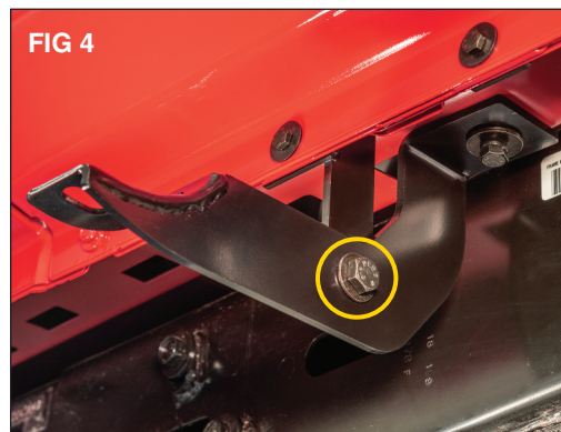
Next align the mounting slots between the two brackets and loosely install a 10mm bolt (A) with washers (G) on both sides and secure with a 10mm nylock nut (E) using a 16mm hex wrench and a 17mm socket. (FIG 4)
