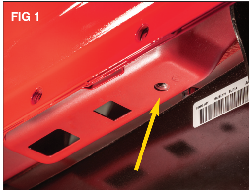
Put on safety glasses. Starting at the front of vehicle locate the vertical threaded hole behind the pinch weld. (FIG 1)
