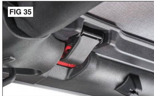
*Please Note: With the rear corners attached the first time you fold down the front header it will be **EXTREMELY TIGHT**. This is normal. We highly recommend that two people fold down the header simultaneously. This will prevent damage to the hardware system.*
