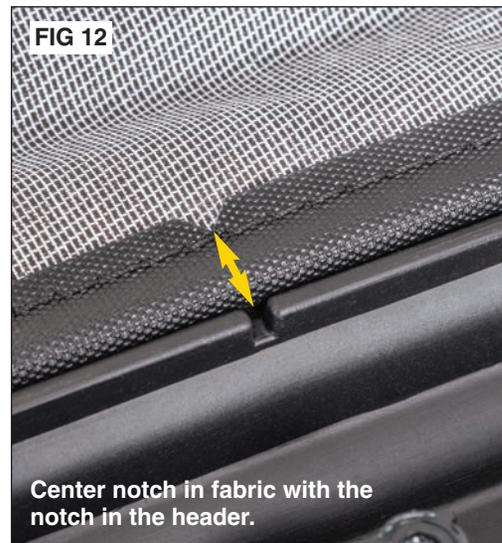
Locate and line up the center notch in the middle of the fabric to the center of the channel centering the fabric on the lower header. Secure the fabric around the center notch with masking tape. See Fig 12.
