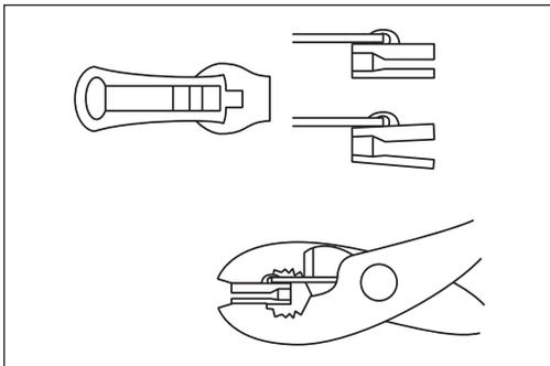
by using an ordinary pair of pliers to bring the sides back into parallel. Return slider to the end of the zipper in the normal Open position. Squeeze lightly at
