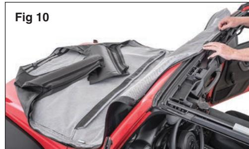
As seen in Fig 10, drape the soft top fabric backing side up over the hood and the windshield and locate the front extrusion sewn into the front header of the Top. Locate the masking tape and have it ready for step 3.
