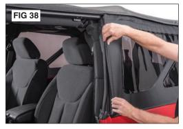
**Step 15: Front of Quarter Windows**Attach the front of the quarter windows along the front edge of the vertical door surround by rolling the plastic into the
