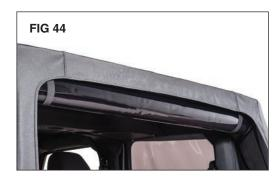
These handy straps can be used to secure your rear window when rolled up. See Figs 43 & 44
