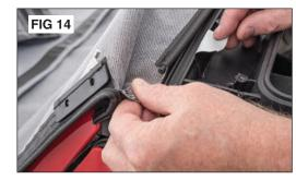
Step 4: Secure Top in Lower Header Working from the center out, secure the top in the lower header channel with masking tape holding it in place for installing the top plate to the lower header. Use 5-6 pieces of tape to hold the top in place. Note: The tape pieces will be completely covered when the top plate is put back on the lower header. See Figs 13, 14 & 15.
