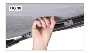
Note that there will **not** be holes in the rear bow fabric/Tabs. You will need to punch the screws through the fabric keeping the top tight while installing. On some models the straps may have to wrap around the opposite side of the bow. Regardless, the bow straps should be tight. See Figs 29 & 30.
