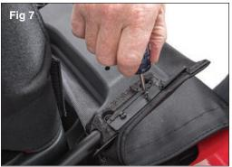
**Step 1B: Remove Existing Top Fabric** Detach your old Soft Top Fabric from the Header. For Model Years 2010-2018 Only: You will need to peel back the corner foam and unscrew the cable attachment on both ends of the header using a T-15 Torx.
