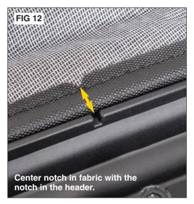
Locate and line up the center notch in the middle of the fabric to the center of the channel centering the fabric on the lower header. Secure the fabric around the center notch with masking tape. See Fig 12.
