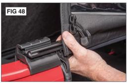
retainer as shown in Figs 45 & 46. After sliding the retainer all the way through the "C" Channel, roll the tailgate bar into the mounts with the outside of the fabric facing towards the rear of the vehicle. See Figs 47 & 48.
