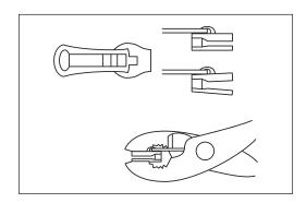
by using an ordinary pair of pliers to bring the sides back into parallel. Return slider to the end of the zipper in the normal Open position. Squeeze lightly at first and test zipper. If the zipper continues to remain open squeeze more firmly with pliers and try the zipper again. Repeat procedure until your zipper operates correctly.
