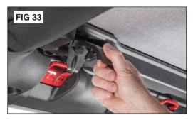
**Step 13: Secure Top Front to Windshield** With the cable spring installed, with two people (one on each side of the header) fold down the header to the windshield and close the front header latches to secure the front of the top to the windshield. See Figs 33-35.
