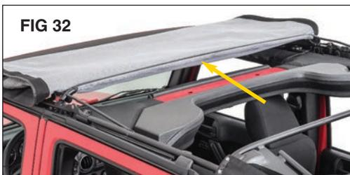
Then, from inside the vehicle, attach the hook and loop flap around the front bow (Bow #1 over the sound Bar). See Fig 32.
