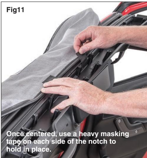
**Step 3: Center New Fabric on Windshield Header with Tape**
