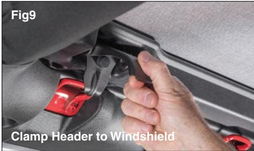
**Step 2: Install the New Top Fabric to the Windshield Header**
