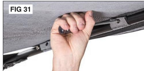
Note that there will **not** be holes in the rear bow fabric/Tabs. You will need to punch the screws through the fabric keeping the top tight while installing. On some models the straps may have to wrap around the opposite side of the bow. Regardless, the bow straps should be tight. See Figs 30 & 31.
