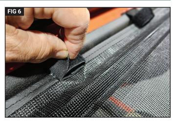
Pull Skylite Sun Shade forward and insert front metal hooks into open hole in the sides of the windshield frame. Repeat for other side (Fig. 5). Secure center hook and loop straps to windshield Freedon Panel tabs (Fig. 6).
