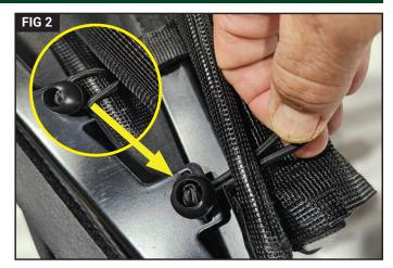
Roll up Skylite Sun Shade panel and secure with hook and loop straps as shown (Fig.1). Remove Bungee retainer from shade and loop the bungee cords through metal mounting tabs on Skylite Roll Back Top. Pull Bungee cord through Skylite Sun Shade grommet and secure to Bungee ball (Fig.2).
