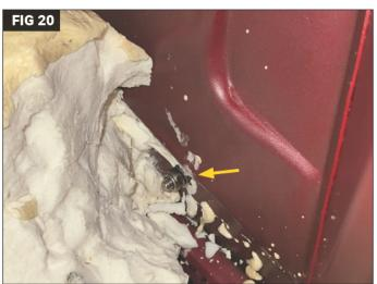
There is foam insulation inside the cavity. Some of this will need to be broken off and removed to access the hole in the very bottom where the rivet came through the wheel well. Place the M6 button head bolt through the wheel well from the outside. (Fig 19) Place the M6 flat washer and nylock nut onto the bolt. Tighten fully. (Fig 20)
