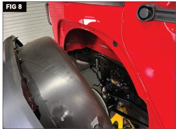
Using even force and hands grasping the edge of the fender flares, pull directly away from the quarter panel. (Fig 7) There will be tension from the clips and you will feel resistance until they release. Some clips my stay attached to the quarter panel. (Fig 8) Remove any clips that stay attached to the quarter panel with a pry tool and reattach to the fender flare.
