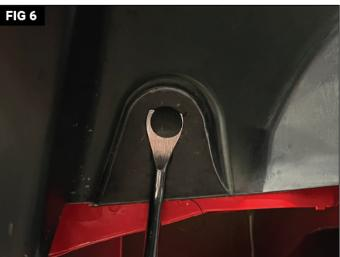
Locate the six plastic retainer rivets. (Fig 5) Using a pry tool, remove each of them and discard. (Fig 6)
