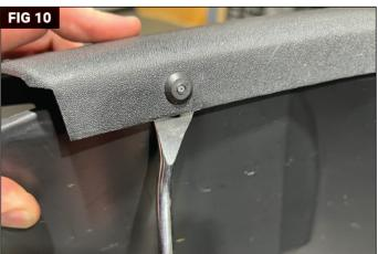
Locate the six plastic retainer rivets that retain the flare to the liner. (Fig 9) Disconnect the inner fender liner from the fender flare by using a pry tool between each piece at the plastic retaining rivets and pry out. (Fig 10)
