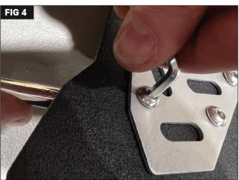
Insert a button head bolt into each hole from the top. Place an M6 flat washer and nylock nut from the back onto each button head bolt. (Fig 3 & 4)
