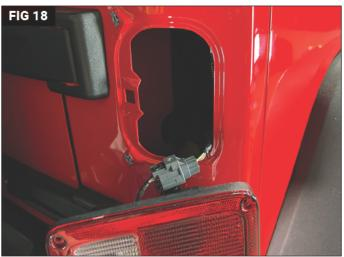
Remove the 2 inside screws (closest to the tailgate) of the rear taillight housing. Keep these for reassembly. (Fig 17) Slide the taillight assembly toward the tailgate and pull away from the body. Carefully rest the assembly against the body. (Fig 18)
