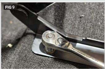
Using supplied M8 Nylock nuts and M8 Flat washers secure riser to Quadratec Seat slider. Tighten all bolts. (Fig 6) Inspect 9/16" mounting threads on vehicle. If needed chase threads with 9/16" tap/thread chaser. Reinstall New Quadratec Seat Riser, seat slider and seat into vehicle using the four (4) riser mounting bolts removed in Step 1. Torque mounting bolts to 34 ft/lbs. (Fig 9)
