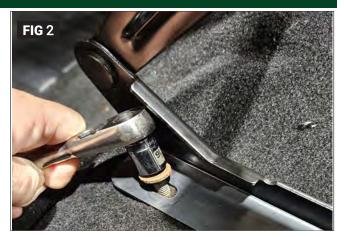
If Original riser has welded on nuts the Quadratec Seat Sliders cannot be used. New seat risers will be required. (Fig 1) Quadratec Seat Riser P/N: 24210-2006 & 24210-2007. If equipped with removable nuts proceed as instructed.
