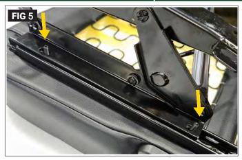
Push down (toward seat bottom) on Quadratec Slider adjuster arm and push inner slide (with mounting studs) back to expose front seat mounting holes. Secure to front mounting hole using bolts removed earlier. Double check adjuster arm function. Tighten all bolts. (Fig 4) Place riser onto seat and seat slider. Riser may need to be pressed at each corner for Quadratec Slider mounting studs to pass through riser mounting holes. (Fig 5)
