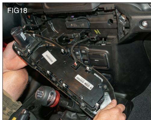
Disconnect any wiring harnesses and set control panel aside. (FIG 18)
