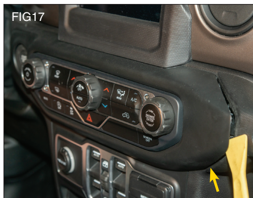
Put on safety glasses. Using a trim clip removal tool gently remove the center dash control center (FIG 17)
