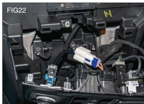
Connect the white connector to the original plug you just disconnected in FIG5. Connect the gray connector back into the 12v socket. (FIG 22)
