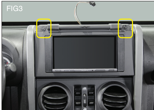
Remove the two upper screws using a 7mm socket. (FIG 3) Using a trim clip removal tool gently remove the lower
