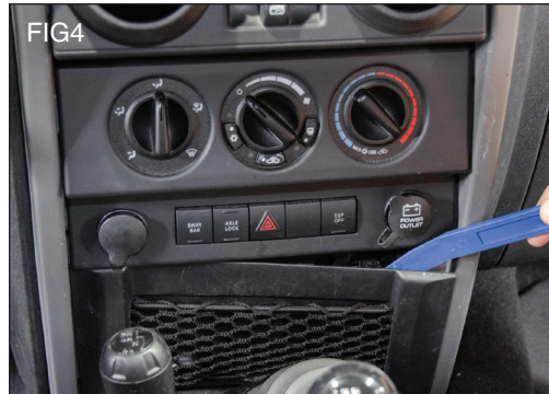
dash panel starting at the top. (FIG 4) There are clips at the top and then it will lift upward and out.
