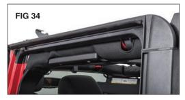
**Step 9B: Secure Rear Over-Door Extrusions**
