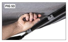
from your original top. On some models the holes in the center bow are in front, on the bottom of the bow or on the rear of the bow. Regardless, attach the bow flap to the bow in the existing holes. See Figs 52 & 53.
