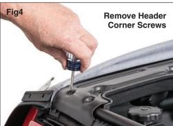
screws (Depending on model year). See Step 1b on next page for proper removal of header fabric. Make sure you keep all screws and fasteners in a safe place after removal. You will be using them again later in the installation.
