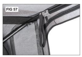
**Step 17: Elastic Window Roll Straps**Snap the elastic window roll straps on the rear bow above the rear window opening as shown.
