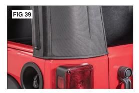
securing the rear corners into the retainers on the vehicle. See Figs 38 & 39
