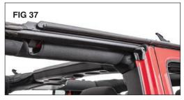
**Step 9C: Secure Front Over-Door Extrusions**
