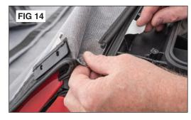
Step 4: Secure Top in Lower Header Working from the center out, secure the top in the lower header channel with masking tape holding it in place for installing the top plate to the lower header. Use 5-6 pieces of tape to hold the top in place. Note: The tape pieces will be completely covered when the top plate is put back on the lower header. See Figs 13, 14 & 15.
