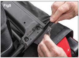
For Model Years 2007-2009 Only: You will need to peel back the foam and remove the two corner screws that hold a plastic mounting flange located in the same vicinity. See Figs 5, 6, 7 & 8.
