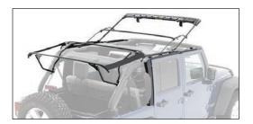
Important: Existing soft top hardware required to install this top. Check to make sure your hardware looks like the picture to the left.
