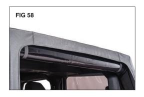
These handy straps can be used to secure your rear window when rolled up. See Figs 57 & 58
