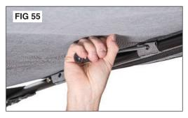
Step 16: Reinstall Rear Bow Screws
