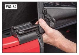
After sliding the retainer all the way through the "C" Channel, roll the tailgate bar into the mounts with the outside of the fabric facing towards the rear of the vehicle. See Figs 61 & 62.
