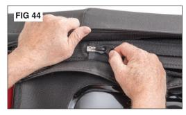
**Step 12: Attach Quarter Window Zippers**Attach the quarter window zippers by starting the zipper on the quarter window and zipping it closed 2-3
