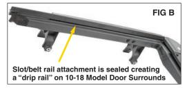
surrounds. If you have an open "slot" found on Fig A, you will need to use the Conversion kit included in 2007-2009 model Soft tops. Please proceed to steps 9A - 9C. If your door surround has this slot filled as shown in Fig B, you can skip the use of a conversion kit and proceed to step 9.
