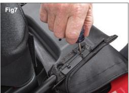
Step 1B: Remove Existing Top Fabric Detach your old Soft Top Fabric from the Header. For Model Years 2010-2018 Only: You will need to peel back the corner foam and unscrew the cable attachment on both ends of the header using a T-15 Torx.
