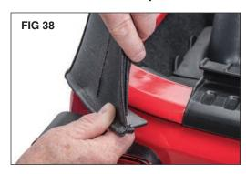
**Step 10: Secure Rear Corners**With the soft top fabric draped across the rear bow and the front header loose, gently pull down on the rear bow while
