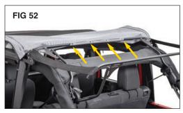
**Step 15: Reinstall Center Bow Screws**Fold the top fabric forward to Expose
