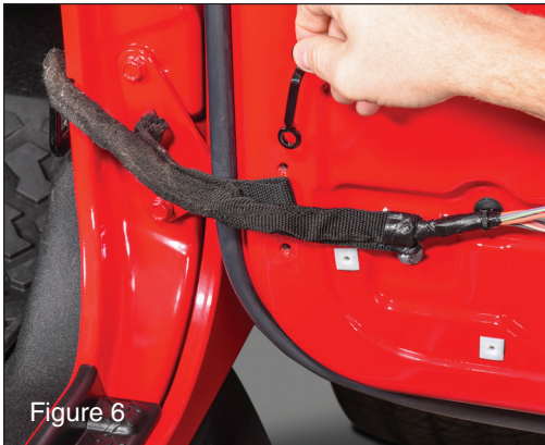
Remove the footman loop from the door and slide it out of the loop on the check strap. (FIG6)
