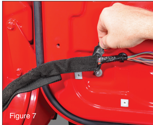
Carefully remove the electrical tape that is attached to the end of the check strap. (FIG7)
