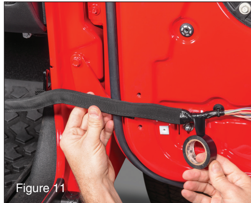
Slide the check strap over to the area of the wiring harness where the original strap was taped in place. Attach the new harness to the wires in the original spot with a few wraps of electrical tape. (FIG11)
