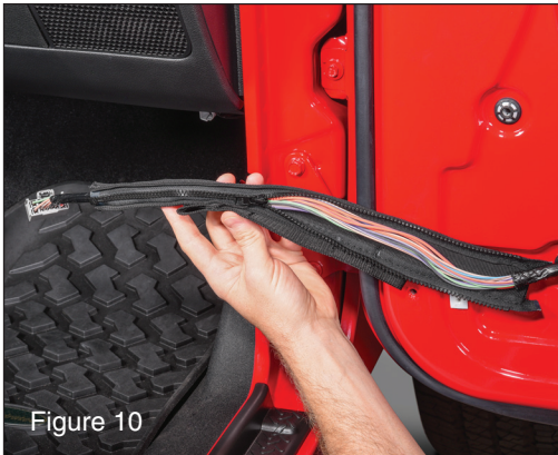
Install the new replacement check strap over the wiring harness and zip the zipper together. The check strap should be installed with the zipper facing down toward the bottom of the harness/door. (FIG10)
