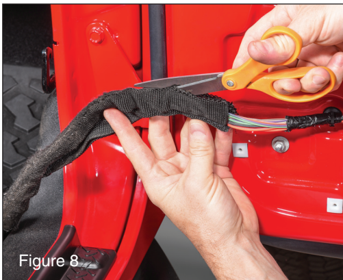
Using a pair of scissors, very carefully cut the old check strap off of the wiring harness. Make sure you do not cut or damage the wires. (FIG8)
