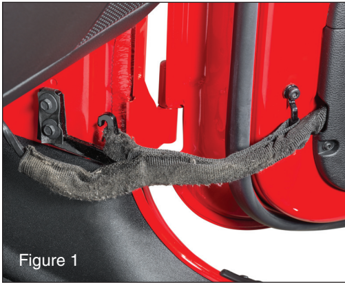
Put on safety glasses. Locate the worn factory check strap. (FIG1)
