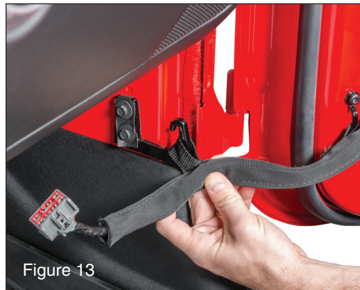
Next, slide the desired front loop of the strap over the factory retaining hook on the kickpanel of the vehicle and reconnect the wiring harness under the dash. (FIG13) Reinstall your door panel. Repeat all steps on opposite side of the vehicle. Your new Quadratec adjustable door check straps are now installed.
