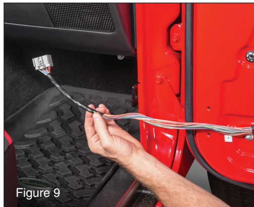
Completely remove the factory check strap from the wiring harness as shown. (FIG9)
