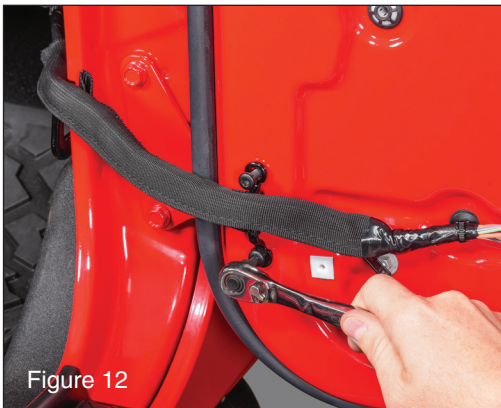
NOTE: These replacement check straps are adjustable at both ends, allowing you to install it in various lengths depending on how far you want your door to open. First, slide the Footman loop through the desired loop on the check strap and reinstall it with the two factory T30 bolts. (FIG12)
