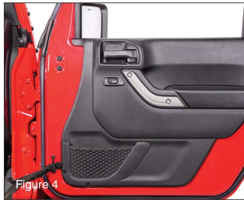
Remove the front loop of the of the check strap from the retaining hook. (FIG3) Then, open the door and be careful not to allow it to open too far. (FIG4) This could cause the mirror to impact and dent the hood cowl.
