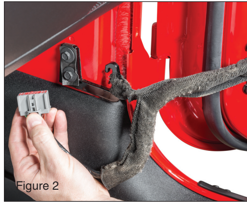
Disconnect the door harness from underneath the dashboard/kickpanel. (FIG2)
