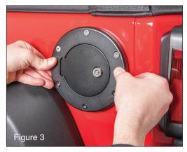
Carefully position the filler door over the filler neck of your vehicle; Taking care to make sure the fuel door is parallel to the ground. Push firmly on the door and hold for 30 seconds to ensure the tape adheres.
