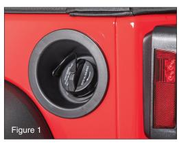
Put on safety glasses. Locate the fuel filler neck on the left rear of your vehicle. Make sure the outside filler neck is clean and free of grease or oils. Cleaning with rubbing alcohol is recommended to promote proper adhesion.
