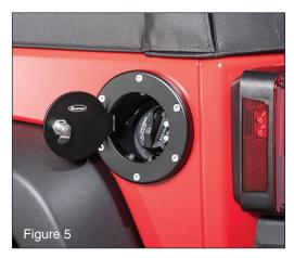
Note: Fuel cap may interfere with the locking mechanism if the cap is left in the horizontal position. If this occurs rotate the cap to a vertical orientation as shown above in FIG5.
