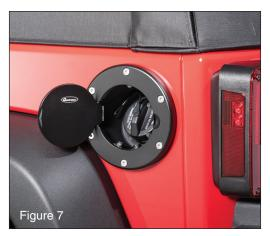
Non-locking style cap installed complete in open door position.
