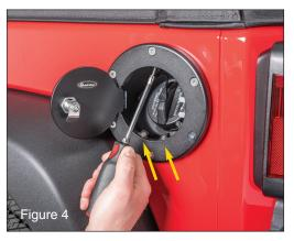
Using a Phillips screwdriver, carefully install the 3 supplied screws. Some force may be required to allow the screws to tap into the plastic of the filler neck.
