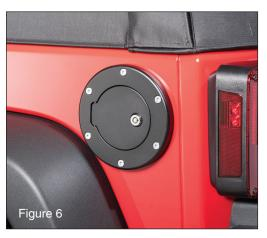
Locking style cap installed complete.
