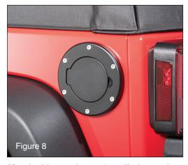
Non-locking style cap installed complete in closed position.
