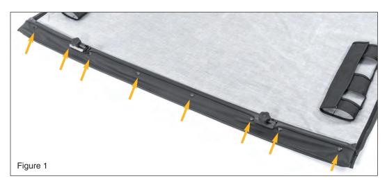
Put on safety glasses. With the windshield header removed from the vehicle, install the front edge of the header into the pocket sewn on your Bimini Top or Bimini Top Plus. Pull the fabric over the header and snap all (8) snaps as shown. (FIG 1)
