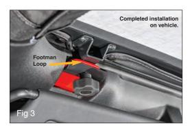
Repeat on the opposite side of the vehicle. Once both knobs are secure, you can continue installation of the Bimini or Bimini plus onto your vehicle. (FIG 3)
