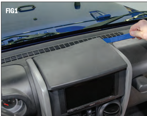
Put on safety glasses. Using a trim clip removal tool gently remove the dash top panel. (FIG1) There are clips at the back and then it will lift off toward the rear of vehicle.
