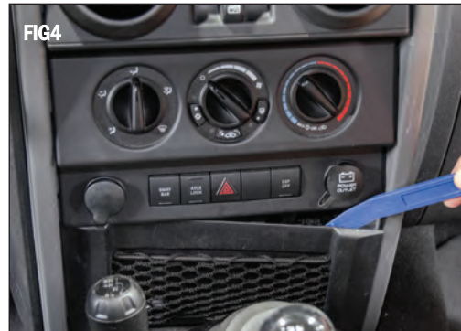
starting at the top. (FIG4) Using trim removal tool pry the top lip and pull upward and out.
