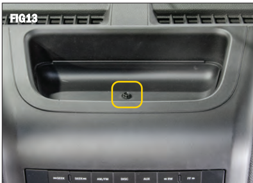
On top of the dash lift up the rubber tray insert and remove the screw using a 7mm socket. (FIG13)
