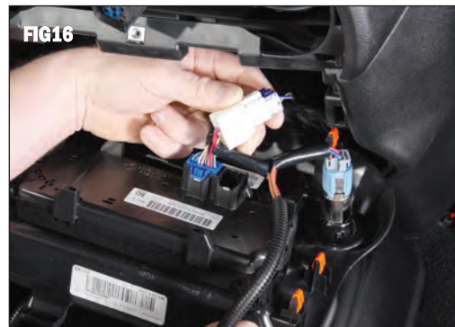
Connect the white connector from the Power Tap Harness to the original plug you just disconnected in FIG 15. Connect the gray connector back into the 12v socket. (FIG 16)
