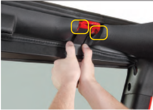
While pulling down on the light brackets, tighten the footman loop screws. (FIG 29)
