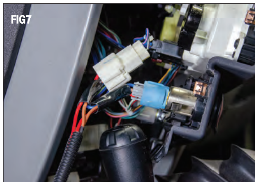
Connect the white connector from the Power Tap Harness to the original plug you just disconnected in FIG 6.
