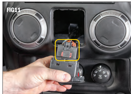
On the window control switch slide the red locking tab over, squeeze the black tab and disconnect the harness. (FIG 11)
