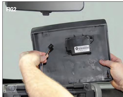
Disconnect the compass module harness from the top panel. (FIG 2)
