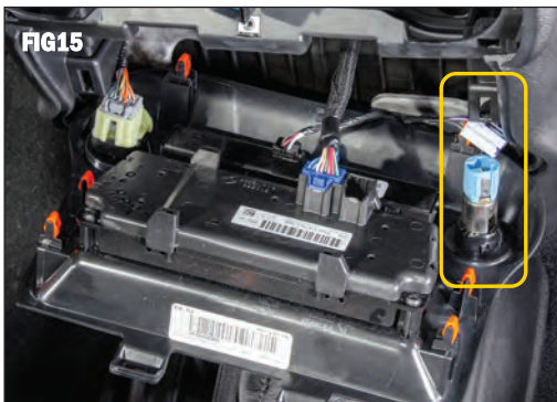
Tilt the panel away enough to access the 12v socket connection. Squeeze the black tap and disconnect it. (FIG 15)
