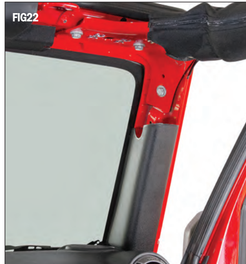
Remove the lower a-pillar trim by pulling from the top. (FIG 22) There is one clip holding it to the a-pillar.
