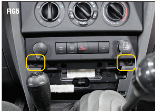
Remove the two lower screws using a 7mm socket. (FIG 5)
