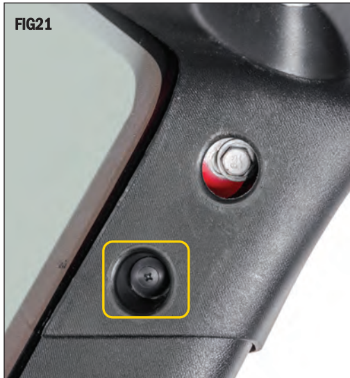
Remove the passenger side a-pillar trim clip using a phillips head screwdriver. (FIG21) Remove the trim panel by pulling downward. It's held into the roll bar by a christmas tree clip.
