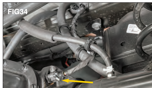
On Rubicon models, slide the gray tab, squeeze and remove the axle locker harness plug. (FIG 34)
