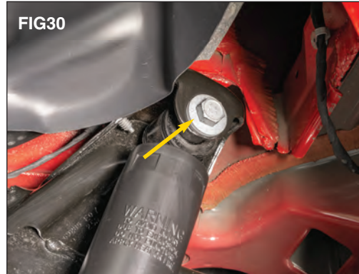
Remove the shocks from the frame using a 18mm socket. (FIG 30) Save hardware.
