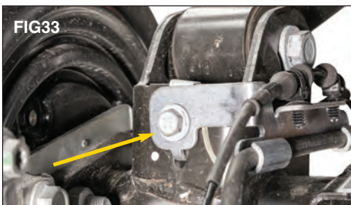
Disconnect the brake line brackets from the upper control arm mount using a 13mm socket. (FIG 33) Save hardware.
