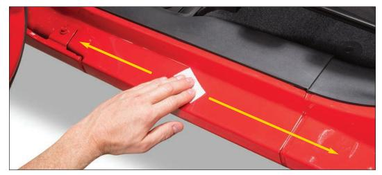
Step 1: Clean threshold contact area with an alcohol prep pad. Remove one alcohol prep pad from its packet and wipe the entire contact area with the
