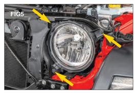
Remove the original headlights using a 10mm socket. Save hardware. (FIG 5)
