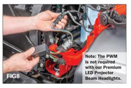
Connect the PWM harness to the JL adapter harnesses, you will hear a "click" when fully engaged. (FIG 8)
