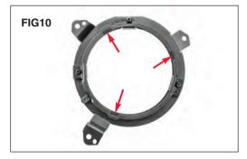
Lay your headlights in place, making sure they are lined up with the notches in the bracket and secure using the trim ring and 3 Phillips head screws. (FIG 10)
