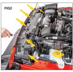
Locate the six plastic fasteners that secure the front grille to the upper body support (FIG 2).
