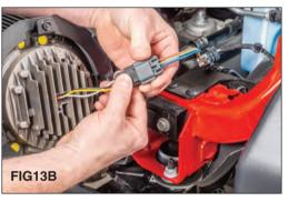
On the Premium LED Projector Beam Headlights you will hear an audible "click" when connector is fully engaged.
