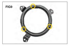
On your new headlight brackets, remove the 3 screws holding the trim ring using a Phillips head screwdriver. (FIG 9)
