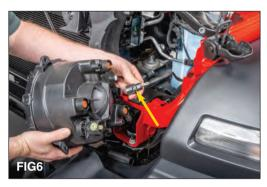
Disconnect the headlights by depressing the black latch & pull outward. (FIG 6)
