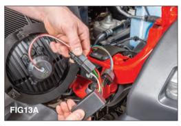
Connect the new LED headlight harness to the other connector on the Pulse Width Modulation (PWM) Harness (FIG 13A) or JL adapter harness. (FIG 13B)
