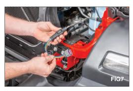
Connect the JL adapter harness to the vehicle harness. You will hear a "click" when fully engaged (FIG 7)
