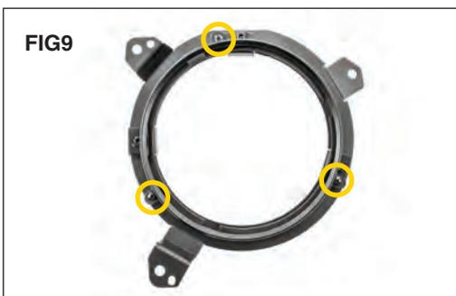
On your new headlight brackets, remove the 3 screws holding the trim ring using a Phillips head screwdriver. (FIG 9)
