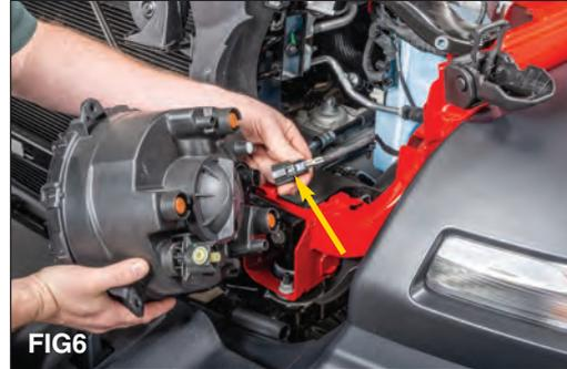
Disconnect the headlights by depressing the black latch & pull outward. (FIG 6)
