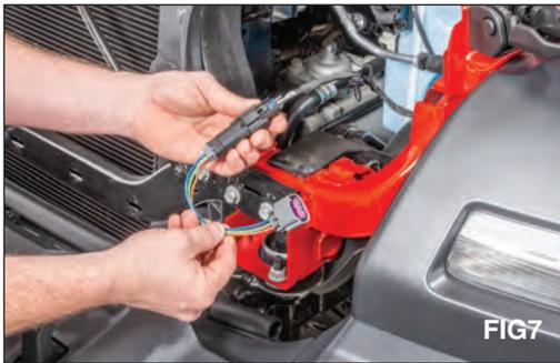
Connect the JL adapter harness to the vehicle harness. You will hear a "click" when fully engaged (FIG 7)
