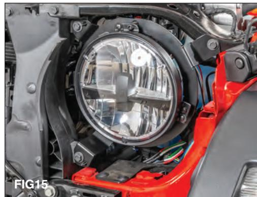
Align the three tabs on the headlight bracket with the vehicle and install using the 3 original bolts. (FIG 13)
