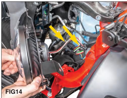
Carefully stow the wiring and or PWM into the headlight bucket area. Be careful not to pinch any wires. (FIG 12)
