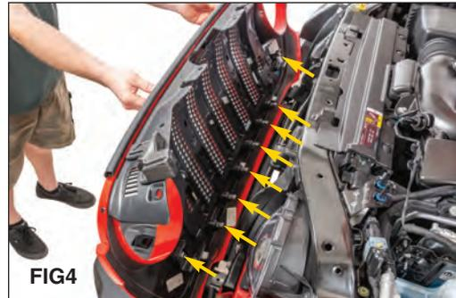
Gently tilt the grille forward and then gently pop the lower portion of grille from its (8) retaining clips. (FIG 4).
