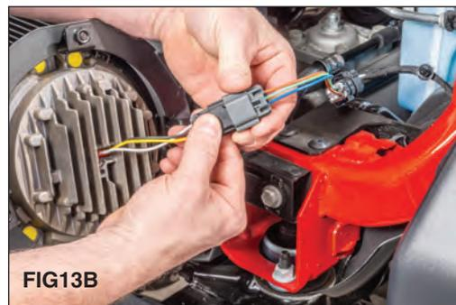
Connect the new LED headlight harness to the other connector on the Pulse Width Modulation (PWM) Harness (FIG 13A) or JL adapter harness. (FIG 13B)
