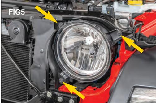
Remove the original headlights using a 10mm socket. Save hardware. (FIG 5)
