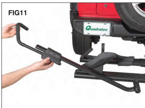
Fold the tire holder arm to the outside of the rack. (FIG11)
