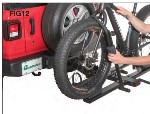
Place the bicycle onto the rack with the front wheel in the tire cradle. Fold the tire holding arm up over the front tire of the bike and pull down on the tire holder until it firmly holds the front tire into the tire cradle. (FIG12)
