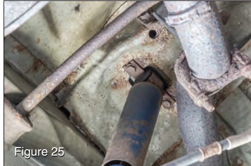
and the top using a 13mm socket. (see FIG 25) Discard rear shocks.
