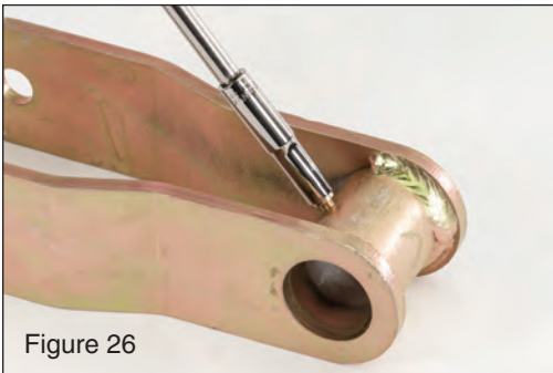
Using a 1/4" socket and hammer, gently tap the grease fitting into the hole drilled in each shackle. (see FIG 26)
