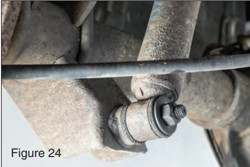
Remove the original shocks at the bottom using a 18mm socket, (see FIG 24)
