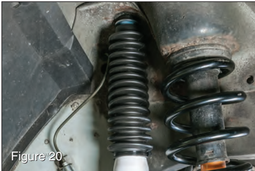
Figure 20 Install front shocks into original opening at top mount and tighten securely a 9/16" socket or wrench. (see FIG 20)
