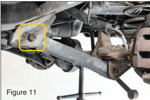
Locate lower control arms and remove frame side bolts using a 21mm socket and open end wrench. (see FIG 11 & 12)
