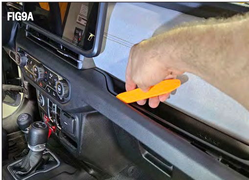
Using trim removal tool gently pry grab handle trim cover and center dash control center away from console. (FIG 9A and 9B)
