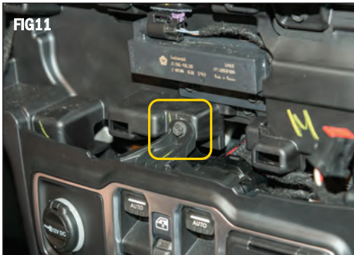
Remove the center screw using a Phillips head screwdriver and set aside. (FIG 11)
