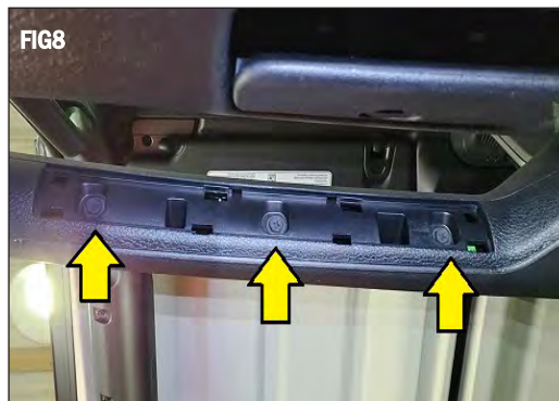
Using the 7mm socket and ratchet remove the three rear facing Phillips head screws. (FIG 8)
