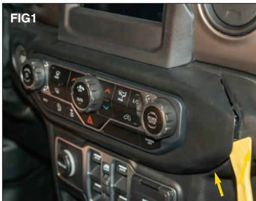
Put on safety glasses. Using a trim clip removal tool gently remove the center dash control center (FIG 1)
