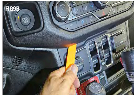
Using trim removal tool gently pry grab handle trim cover and center dash control center away from console. (FIG 9A and 9B)
