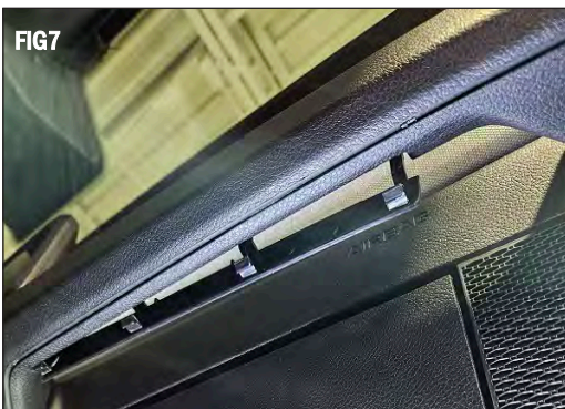
Using trim removal tool pop off screw access panel located on back side of grab handle just in front of glove box. (FIG 7)
