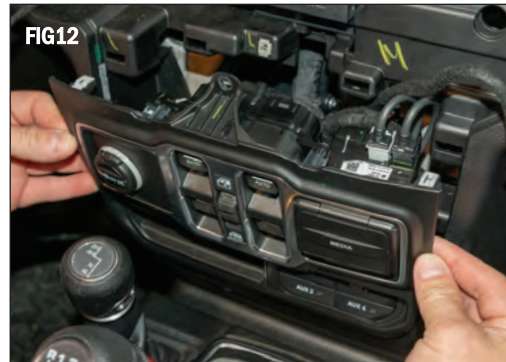
Gently pry out the window control panel from the top and work your way down. (FIG 12)
