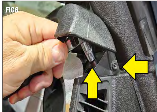
Remove top two grab handle mounting screws using the 7mm socket and ratchet. (FIG 6)
