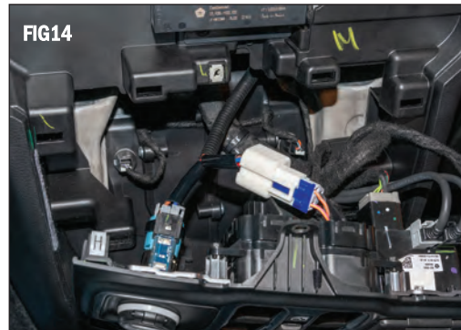
Connect new Power Tap Harness white connector to the plug you just disconnected in FIG14. Re-connect the new Power Tap gray connector back into the 12v socket. (FIG 13)
