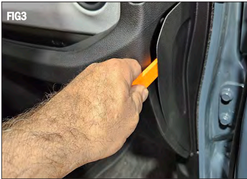
Pop off passenger side cover plate using trim removal tool as shown. (FIG 3)
