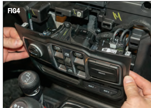
Gently pry out the window control panel from the top and work your way down. (FIG 4)
