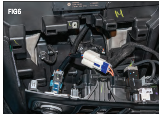
Connect new Power Tap Harness by connecting the white connector to the factory plug you just disconnected in FIG6. Connect the Power Tap gray connector back into the 12v socket. (FIG 5)
