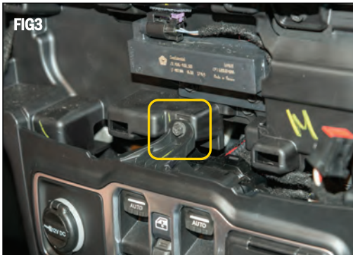
Remove the center screw using a Phillips head screwdriver and set aside. (FIG 3)
