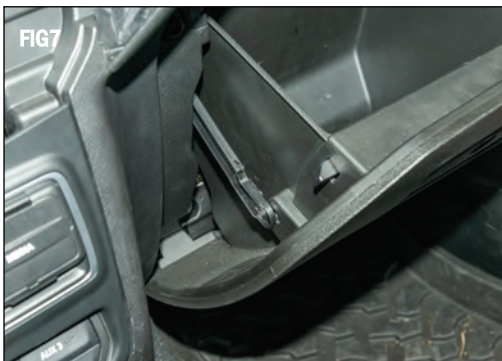
Tilt panel away enough to access the 12v socket connection. Squeeze the blue tab and disconnect it. (FIG 5)
