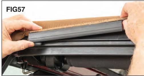
Locate the two plastic strips sewn to the sides of the top above each door (FIG57).
