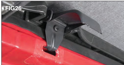
Pull the top down to engage the header clamps on each side of the windshield
