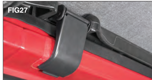
and secure the Header to the windshield (FIGs 25, 26 & 27).
