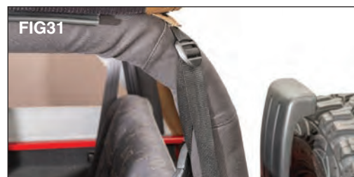
(FIG30). Repeat this on the other side of the vehicle and while pulling towards the rear of the vehicle, tighten one strap and then the other side strap tightening up the top deck. Do not tighten completely (FIG31).
