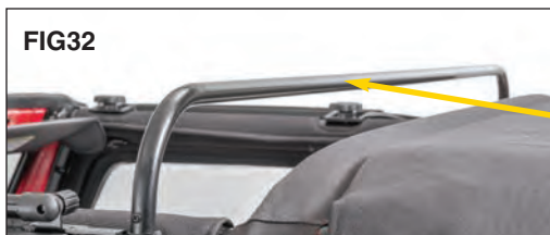
IMPORTANT: The top deck MUST be centered on the rear of the vehicle for the windows to fit properly.
