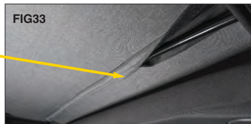
Once the rear straps are secure (but not tightened all the way), go inside the Jeep and make sure the center bow flap is wrapped round and secured to the center bow. Also double check to make sure the safety strap shown in Fig 21A is looped around the center bow (FIGs 32 & 33).
