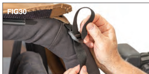
Once the front header is secured, go to the rear corner of the Top deck and locate the rear corner straps. Thread the straps down and under the seat belt mount as shown in FIGs 28 & 29 and thread the strap through the buckle
