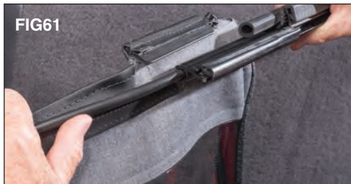
Slide the "C" shaped channel onto the tube sewn into the rear window with the round seal down. See FIG61 for correct alignment. Slide the tailgate bar all the way across the rear curtain.
