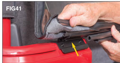
Open the rear tailgate. As shown in FIG41, insert/roll the tailgate bar into the mounts on each side of the tailgate with the vinyl side of the rear curtain facing the rear of the vehicle.
