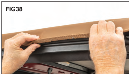
above the door opening (FIGs 37 & 38). Secure the strips on each side of the
