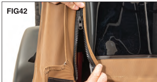
Once the Tailgate bar is secure, lower zippers on both sides of the rear curtain
