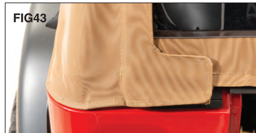
(FIG42) and then secure the rear zipper cover flap as shown in FIG43.
