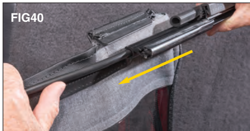
Slide the "C" shaped channel onto the tube sewn into the rear window with the round seal down. See FIG40 for correct alignment. Slide the tailgate bar all the way across the rear curtain.
