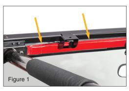
Put on safety glasses. Place the windshield header assembly on top of the rubber seal along the top of the windshield. (FIG 1)
