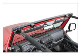
Once both bolts are secured, you are now ready to install your Quadratec Bimini Top accessory directly to the attached windshield header. (FIG 4)
