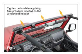
While applying firm forward pressure, tighten the two 5/16" bolts using a ½" wrench or socket and driver. For best results tighten one side ¾ of the way and then tighten the other side ¾ of the way. Then fully tighten both sides making sure the header is completely secure (the header does not move under pressure). (FIG 3)
