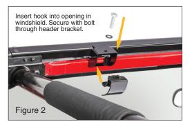
the hook bracket with the top hole in the header assembly. Insert the 5/16 x 1-11/4" bolt and one 5/16" washer from the top into the hook bracket securing the hook bracket to the windshield assembly as shown above. Hand Tighten.
