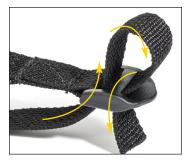
Throughout the installation, you will need to thread webbing straps through buckles several times. Please review the picture for correct strap routing through the buckles. As a rule of thumb, run the strap below and through the sewn side of the buckle first and then back down through the end of the buckle. Tighten the strap by simply pulling the exposed webbing after threading the strap through the buckle.
