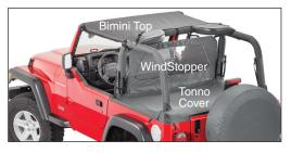
The WindStopper is a great way to stop air flow into the Cab when driving without a soft top. This WindStopper is ideally designed to be used in combination with our Bimini Top/Bimini Top Plus and the Tonno Cover to create the ultimate summer cab top combo. Please note that this product
