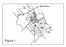
Put on safety glasses. Use the included self drilling Tek Screw to attach the bracket onto the rear frame member at the location of your choice. We recommend towards the center of the tailgate on the driver side. NOTE: An optional clamp is included for installation in other areas of the vehicle, use as desired (Fig 2).
