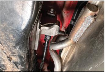
With the Exhaust supported, extract the four (4) 13mm hanger bolts from the factory Exhaust hanger mounts located on the frame (there are two (2) on each side of the muffler assembly), remove the muffler Assembly.
