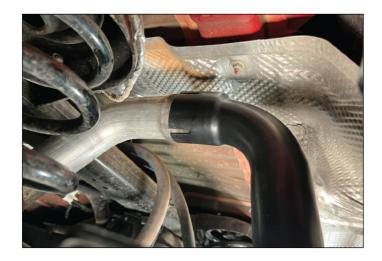
Re-install the Quadratec Exhaust Assembly, by first sliding the inlet over the factory exposed factory outlet Exhaust pipe making sure to a line the Factory Exhaust
