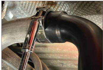
Continue by re-installing the 4 factory 13mm bolts into the factory Exhaust Hanger brackets. Keep all clamps and fasteners loose until final adjustment. Once a final position has been chosen for the new exhaust system, tighten the supplied band clamps must be VERY tight to properly align the pipes and prevent leaks (Approximately 40ft-lbs). Inspect all fasteners after 25-50 miles for operation and re-tighten if necessary.
