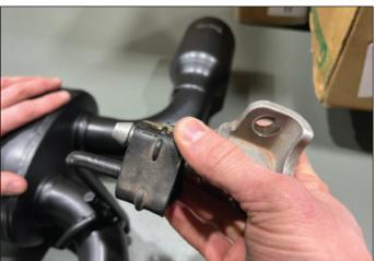
Separate the Rubber retainers and brackets from factory exhaust assembly. Next keeping Left and Right sides orientation in mind transfer the Factory Rubber Retainer Brackets to the New Quadratec Exhaust assembly.
