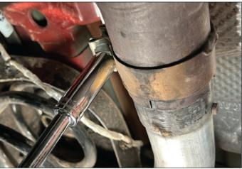
Put on Safety Glasses. Remove the Factory Exhaust system, first locate the clamp in front of the rear Exhaust Assembly, located above the rear axle/sway bar, and loosen with 15mm socket.
