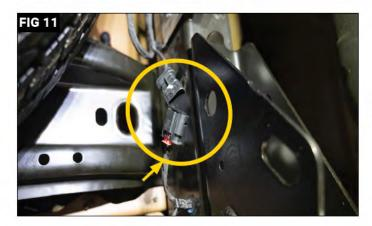
Reconnect the license plate plug and return the red locking tab to secure in place. (FIG 11)
