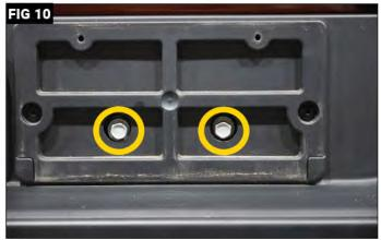
Reconnect rear bumper by reversing your steps in figures 3 and 4. Once rear bumper is set into position, secure with the two (2) bolts on either end of bumper and the two (2) bolts located behind the license plate with a 16mm socket wrench. (FIG 9 and 10)
