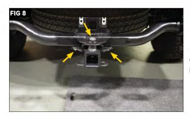
Tighten the M18 x 2.0 x 50mm bolt to 320 lb-ft and the M12 x 1.5 x 40mm Flange Nuts to 110 lb-ft. (FIG 8)
