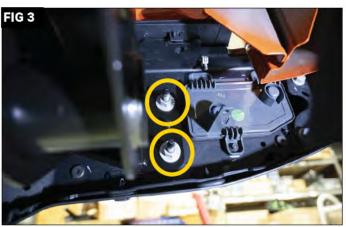
Remove license plate and locate the two (2) bolts. With a 16mm socket wrench, remove the two (2) bolts. (FIG 2) Locate the two (2) nuts at either end behind the bumper and remove with 16mm socket. (FIG 3)
