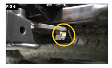
Raise and align hitch receiver into position. Thread the M12  $\times$  1.5 Flange nut carefully onto carriage bolt as not to push bolt back through hole, and loosely secure. (FIG 6) Repaeat on oppostie end.
