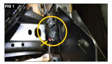
Put on safety glasses. To access the rear crossmember, remove the rear bumper. First, locate the license plate light wiring plug at the rear driver's side of vehicle and disconnect. Pull out the red locking tab of connector followed by separating the black plug. (FIG 1)
