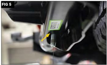
Pull wire back through slowly, pulling Carriage bolt into hitch mount bolt hole. (FIG 5) Carefully remove wire from carriage bolt and repeat on opposite end.
