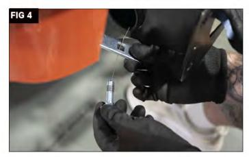
Using the supplied Fishing wire, feed the coiled end of fishing wire through hitch mount bolt hole beneath, and pull toward either end of the rear cross member. Feed the fishing wire through Square hole spacer and then thread the M12 x 1.5 x 40mm Carriage Bolt into wire. (FIG 4)
