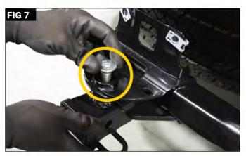
Place the M18 x 2.0 x 50mm bolt through hole in cross member and thread into the hitch receiver. (FIG 7)
