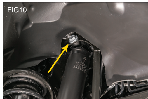
Remove the shocks from the frame using a 18mm socket. (FIG 10) Save hardware.
