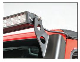
Install washer, split washer, and nut (supplied with lightbar) on both sides.
