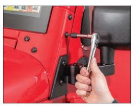
Remove both bolts using a T40 Torx bit and ratchet. Retain bolts for reassembly
