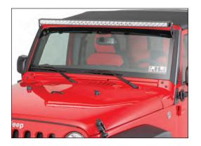
Adjust lightbar to the desired angle, then and tighten the nuts with a 13mm wrench.
