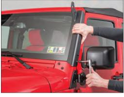
Place the bracket over the hinge plate and align the holes on the bracket with the holes in the factory hinge plate. Reinstall the two T40 torx bolts lightly with at T40 torx bit and ratchet but do not fully tighten at this time.
