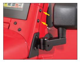
Put on Safety Glasses. Locate the two upper T40 torx bolts on both of the windshield hinges.
